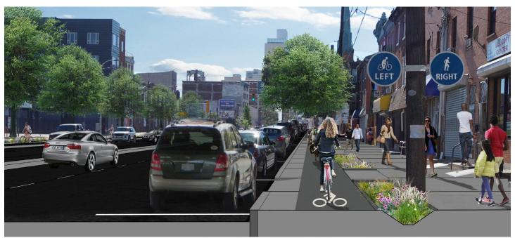
The rendering of a parking-protected raised bike lane on Spring Garden Street shows how improved infrastructure could make the corridor safe for cyclists travelling between the Schuylkill River Trail and the Delaware River Trail, for pedestrians shopping and working on the corridor, and for vehicles that can move more efficiently.
